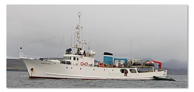
The Expedition will use the vessel Braveheart, owned and operated by Nigel Jolly. The vessel is an ice-strengthened polar research and supply vessel, extensively used for oceanographic touring, research, and amateur radio expeditions. The ship Braveheart accommodates 14 passengers and a crew of five.
