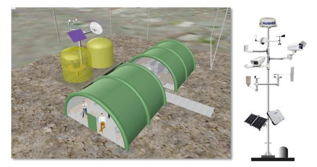
In operation, the controller would accumulate data from the various sensors and inputs, including images from video cameras, and store them for timed or triggered telemetering. In addition, we would provide for the ability to upload instructions for the controller, such as repositioning the camera, changing the interval between image captures, recalibration to aging, and storage management. We believe this system could operate unattended for 5 years or more.
