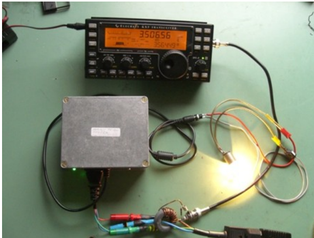
Figure 45: Built-in power supply in a metal housing and Schurter filter. The result: absolutely no interference can be detected with the KX3.
