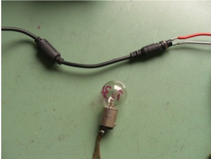
Figure 12, The end of the supply cable is equipped with a suppression choke
