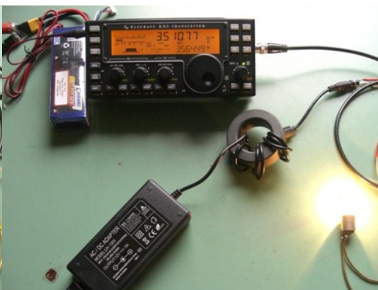
Figure 11, gray ferrite core, FT140A-43
