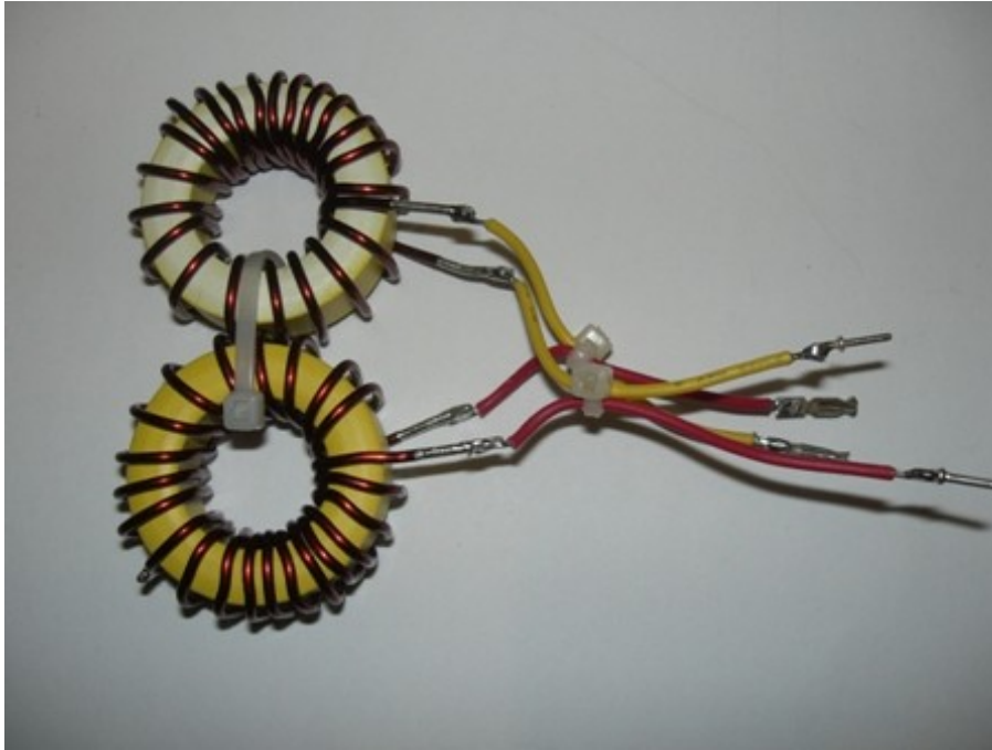
Figure 36, push-pull choke (Gt-Dr) distributed over two cores.
