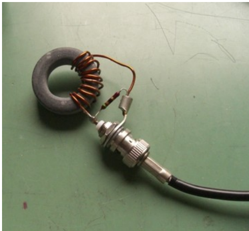
Picture 19, a self-built 50Ω-measuring head
